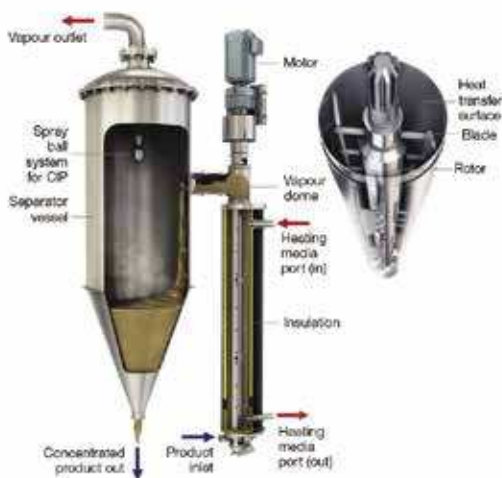
A Contherm unit for pre-heating (left) and a ConVap vapour dome (middle) with separator vessel (right) for evaporation.
