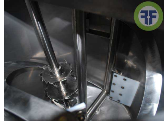
DUAL SHAFT SANITARY MIXING SYSTEM - INTERIOR
