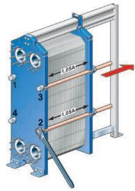
Step 2: Loosen the two diagonal pairs of bolts are loosened alternately, as shown in the figure below.
