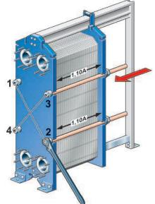
Step 2: After that bolts are tightened alternately and diagonally, as shown in the figure below. Check the dimension A during tightening at the positions of the bolts that are being used.
