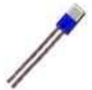
Thin-film RTD element potted in probe with thermally conductive paste
