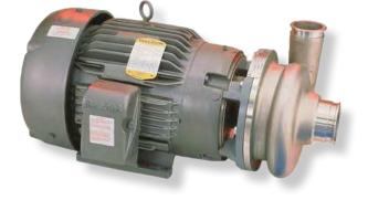
The DV Series, with a unique double volute design, is ideally suited for CIP return applications. The double volute design reduces air binding without an air relief valve at half the cost of a self-priming pump.
