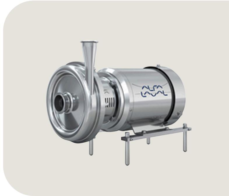
As standard, the LKH pump is equipped with a single mechanical shaft seal but is also available with a single flushed or a double mechanical shaft seal. The front-loading shaft seal, with the spring and washers mounted on the atmospheric side, makes maintenance fast, easy and inexpensive. It takes just a few minutes to replace the shaft seal. In addition, the balanced design minimizes the risk of seal opening during unforeseen pressure shock.
