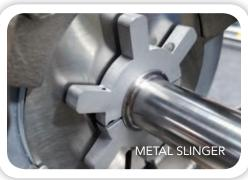
Optional metal slinger is more durable than rubber slingers and dissipates heat away from the motor Hot Oil M Series pumps are modified to make them ideally suited for use in hot (dirty) oil applications. Currently we offer this on the MC3 2 x  $1\frac{1}{2}$  and MC3  $2\frac{1}{2}$  x 2.
