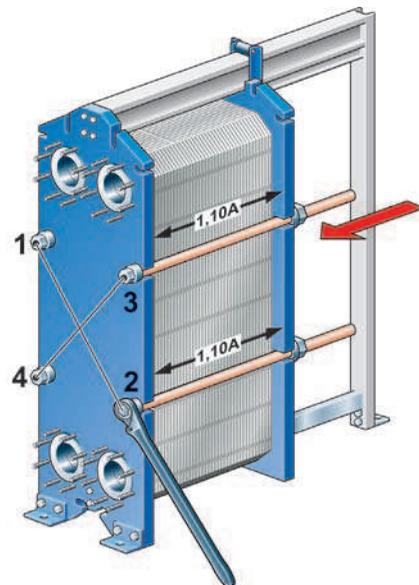
Step 2: After that bolts are tightened alternately and diagonally, as shown in the figure below. Check the dimension A during tightening at the positions of the bolts that are being used.
