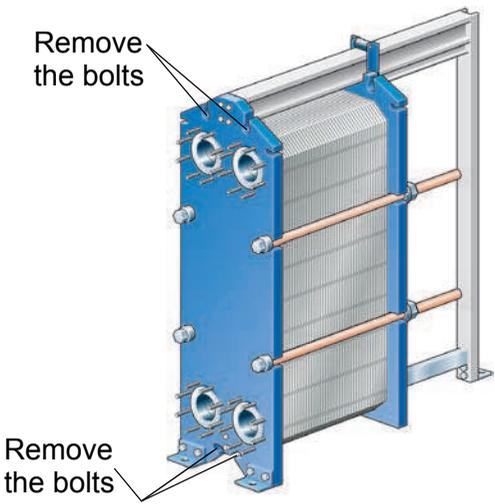
**6** The pairs of bolts that are fitted with bearing boxes are opened alternately and diagonally in two steps, see figures below.
