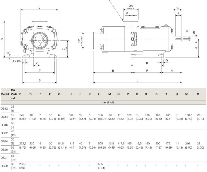
$<sup>^{1}</sup>$  Dimension 'V'is with flush plugs installed - NPT adaptors will increase this dimension by  ${\scriptstyle \sim}10\text{mm}$
