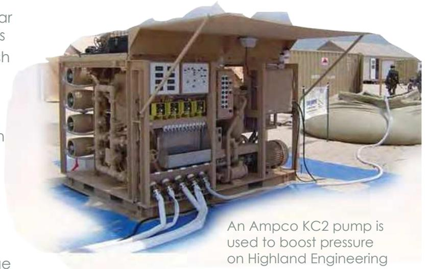
An Ampco KC2 pump is used to boost pressure on Highland Engineering Inc.'s 1500 ROWPU system
