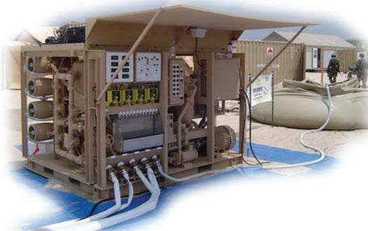
KC2 pumps are used to boost pressure on Highland Engineering Inc.'s 1500 ROWPU system
